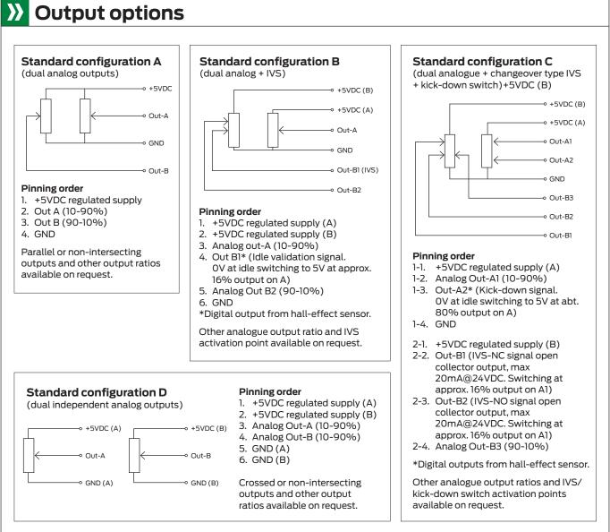
**Cable/ harnessing:** Standard 0.5m PUR insulated cable, flying leads. 6 cores size awg 20. With connector Deutsch DTM or DT 4/6-way (male) as option, other types available on request.
